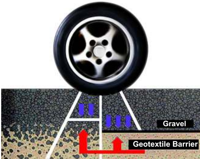
Figure 3: Close-up view of a woven geotextile fabric showing how it reduces the impact of a localized load, and redistributes the localized pressures
